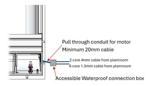
1 x 2 core 4mm cable (for runs under 25m) will be needed to run from this poolside connection deck box to the main Covrex Control Panel in the plantroom.
