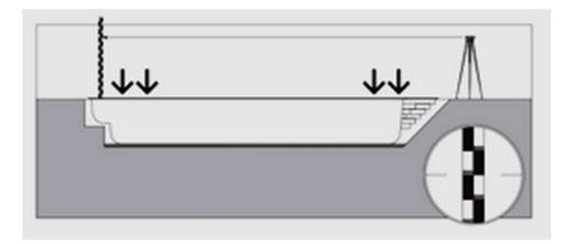
Note: It is important the shell is perfectly level on all four corners, across the sides and back.
