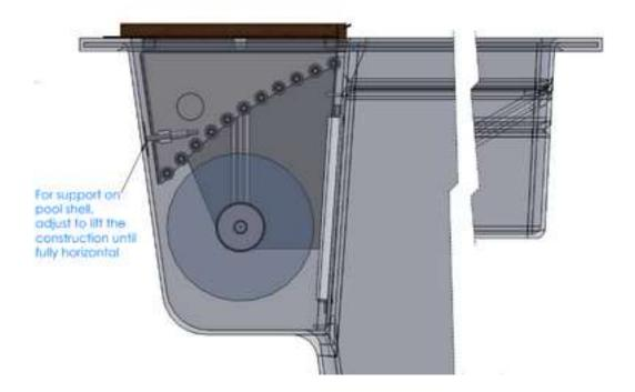
Once the correct level is achieved they should be locked in place by tightening the retaining nut.
