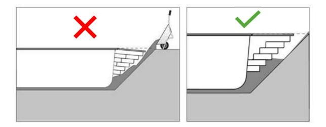
Once these areas have been back filled the remaining area around the pool can be filled. The backfilling material can be pumped around the pool or introduced using a wheel barrow and spade.
