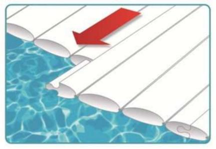
Once all of the slats are on the pool each 800mm section has a small security screw inserted to prevent the slats from sliding when floating on the water as below.
