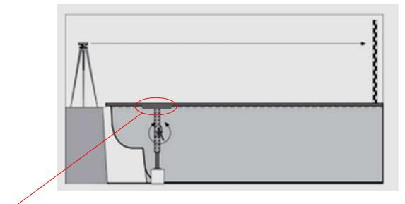
Note: Do not use a singe point of contact if using a jack, instead use a block of wood/hard material to spread the load in the shell.
