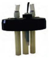
Access to the electrodes is by unscrewing the top ring flange of the chamber and gradually easing out the transparent lid with a screw driver. A rubber 'O' ring situated round the edge of the lid creates a seal. Once the lid has been removed the electrodes can be checked and replaced if necessary.
