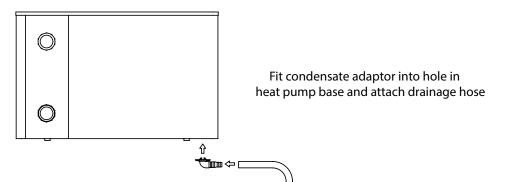
Components are secured to the heat pump base with screws or bolts, and while every effort is made to seal these fittings, small amounts of condensation may still leak through the base.
