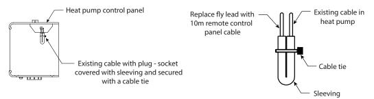
Position the remote control panel mounting box and feed the 10m cable through the appropriate opening. If the cable is concealed within the wall and routed through the rear of the mounting box, use a grommet to protect the cable. Connect the cable to the remote control panel's fly lead, then secure the panel in the mounting box.
