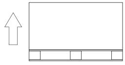
Never lift the heat pump using the water inlet and outlet connectors as this may damage the titanium heat exchanger in the heat pump.
